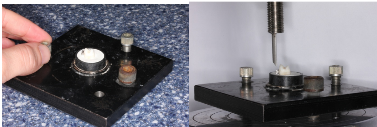
Figure 1: Mounting jig used to provide parallelism between the bracket and the upper member of the Instron testing machine
